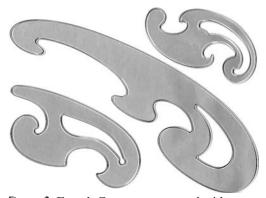
Figure 6. French Curves constructed with elliptical, hyperbolic, and parabolic sections
