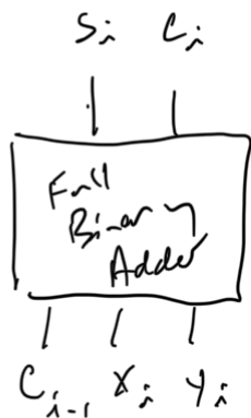
Figure 1: The full-adder takes input digits x_i and y_i , as well as the carry digit c_{i-1} from the previous step and computes write digit s_i and carry digit c_i . Then do it again!
