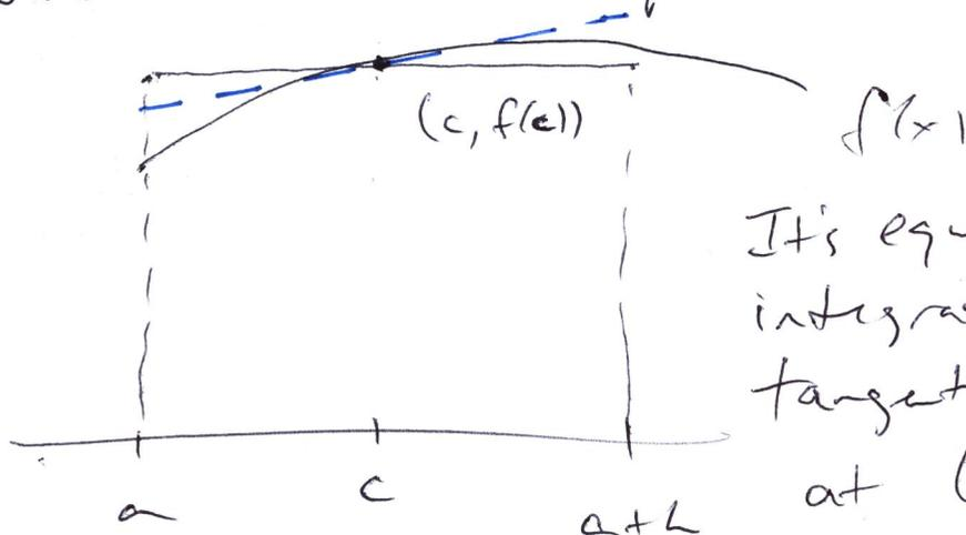
It's equivalent to integrating the target function at  $(c, f(c))$
