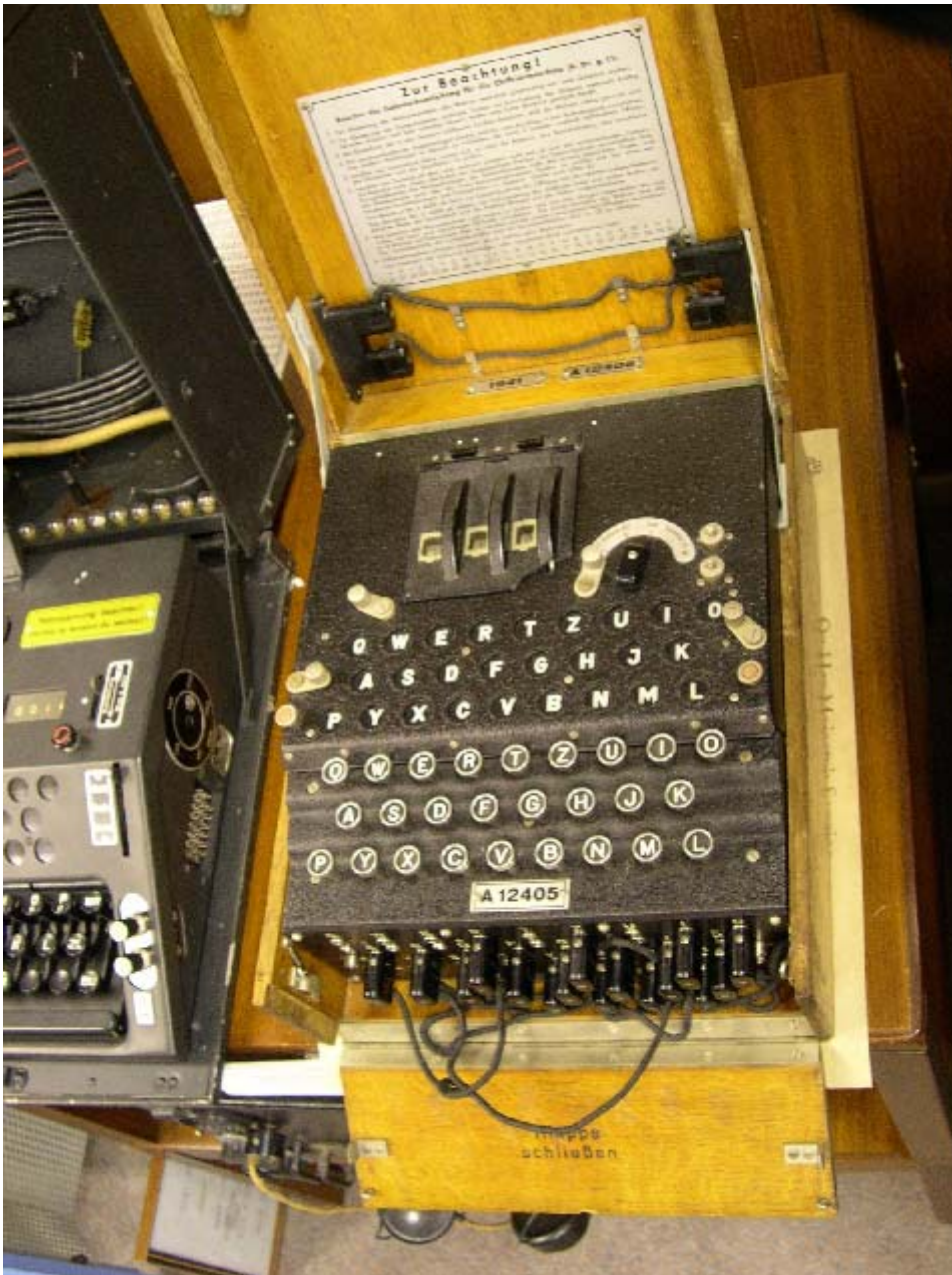
A 3-rotor Enigma machine. The plugboard is at the bottom of the picture. The keyboard is above the plugboard. The lampboard is above the keyboard. The three rotors are under the windows at the top of the picture. Display at the British Intelligence Museum Chicksands.
