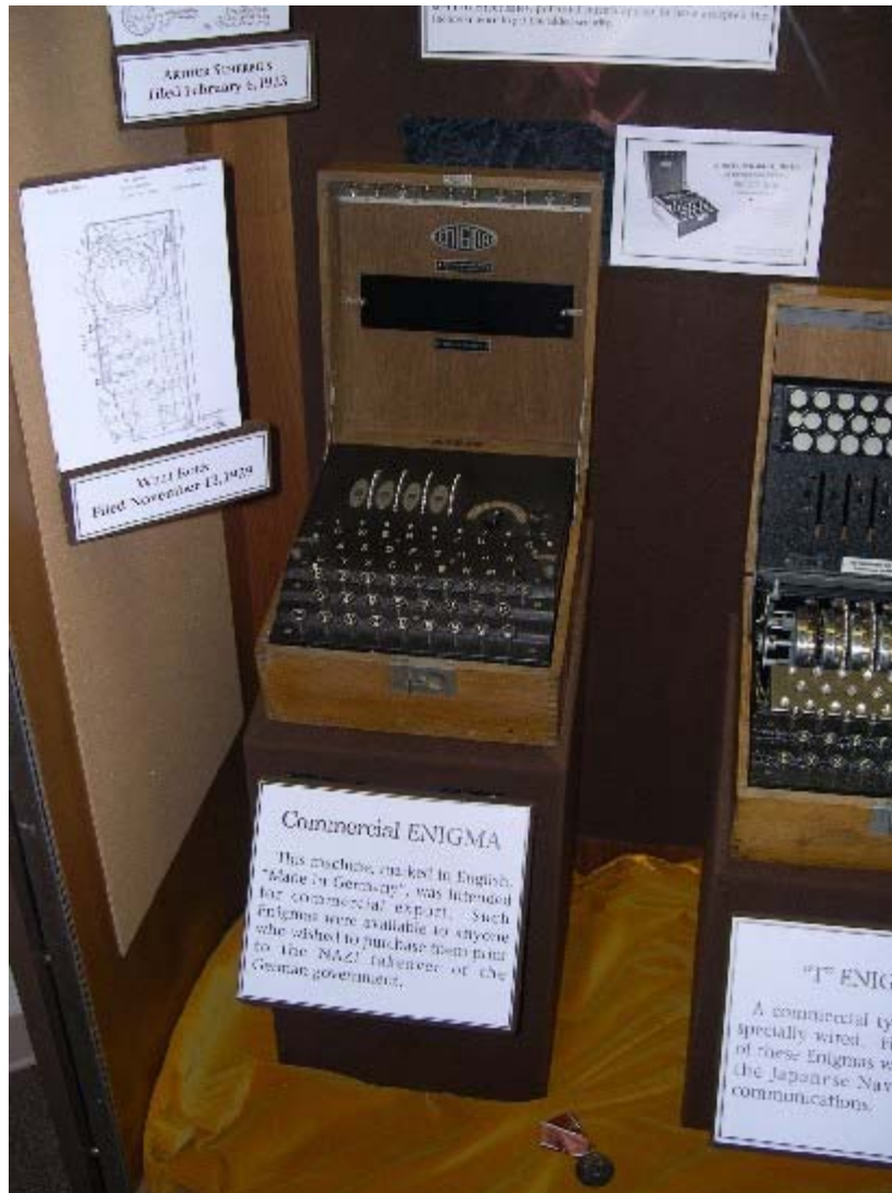
A commercial Enigma on display at the NSA's National Cryptological Museum. Notice that this machine does not have a plugboard.
