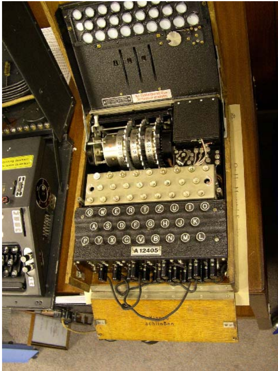
The same Enigma machine with the top open revealing the three rotors and the lamps. Display at the British Intelligence Museum Chicksands.
