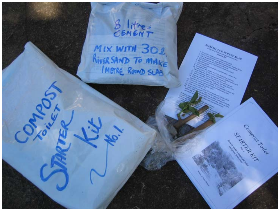
The Compost Toilet Starter Kit is made up of 8 litres of cement packed in its own bag which will make a one metre diameter concrete slab when mixed with river sand and water. The Kit also includes simple instructions for making the concrete slab and an instruction manual for the construction and use of the Arborloo and care for trees. The two young trees are also included.
