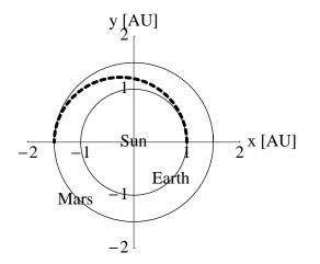
The satellite orbit must have perihelion  $r_{-} = R_E$  (= radius of Earth's orbit) and aphelion  $r_{+} = R_M$  (= radius of Mars's orbit) as shown in the figure. The planetary orbit radii are
