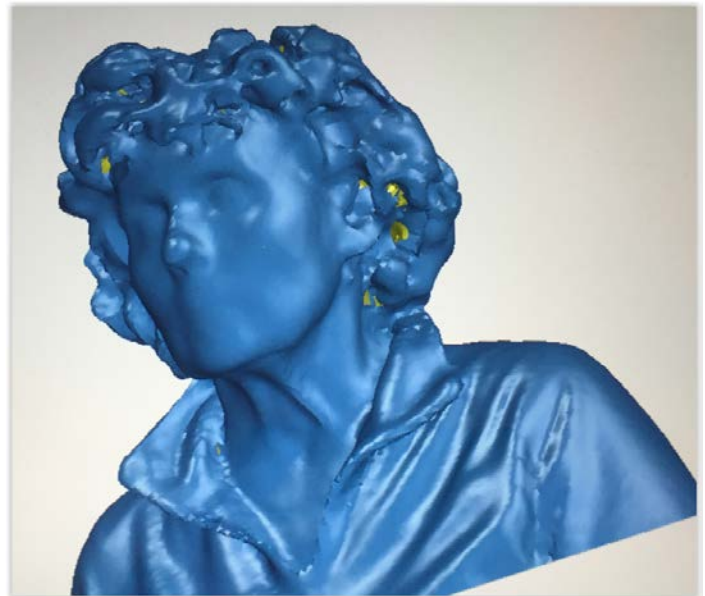
Fig. 1: A typical image scanned by iSense™ 3D scanner being examined for processing by the iSense Software from 3D Systems™ (Rock Hill, South Carolina, USA). As the scan proceeds the holes shown in green get filled (Image is courtesy of Evan Valentine).
