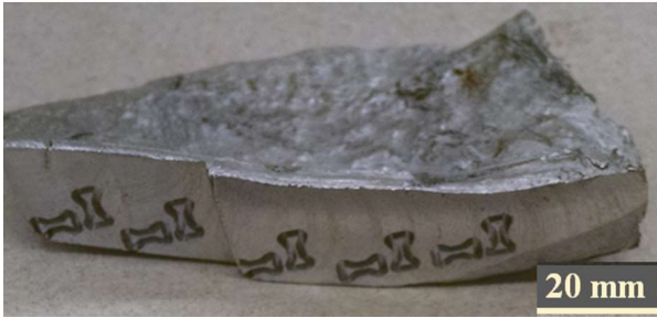
Fig. 6 – Carving dog bone shape samples in covetic aluminum
